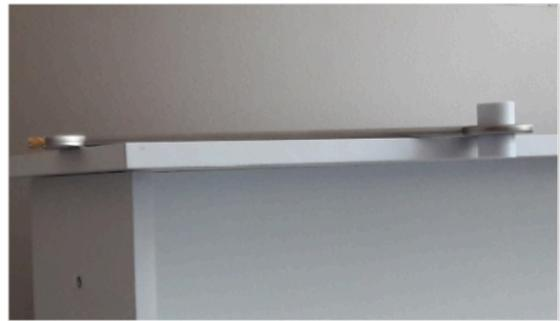
Figure 4.24: Free space directional D-dot probe a), Free space directional B-dot probe b).
