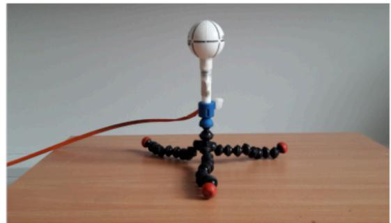
Figure 4.23: Isotropic autonomous electric and magnetic field probe a), electric field probe with optical transmission of signal and power b).
