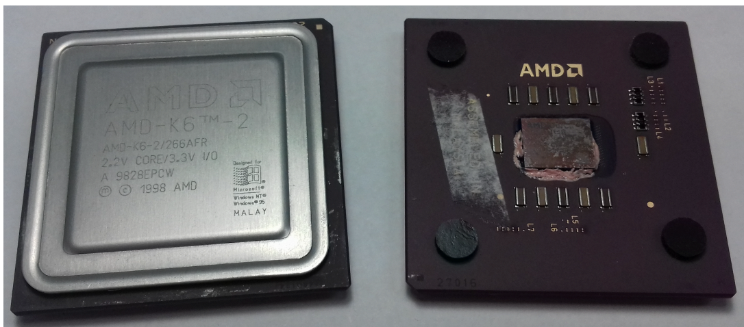
Figure 2.2: Exemplary x86 processors from the turn of XX th century with protective metal shield (AMD K6) and opened with the core exposed (AMD Duron).
