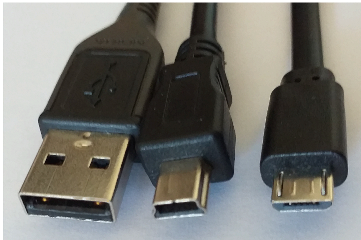
Figure 3.2: Popular USB 2.0 connectors – from left to right: Type A, Type B mini, Type B micro.
